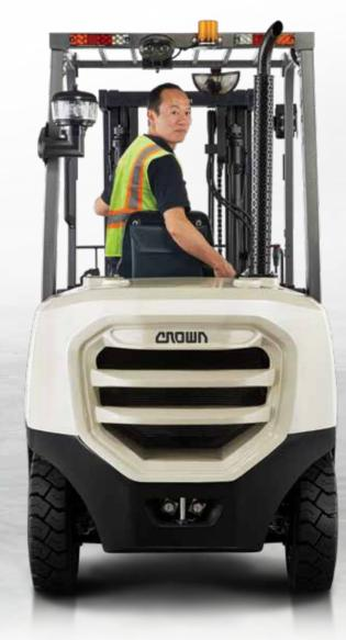
**Counterweight Design** Counterweight design increases airflow and cooling capability in hot climates.
