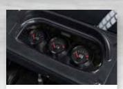
**Instrument Panel** Easy-to-read instrument panel displays coolant and transmission oil temperatures, fuel level, operating hours, oil pressure and alternator voltage.
