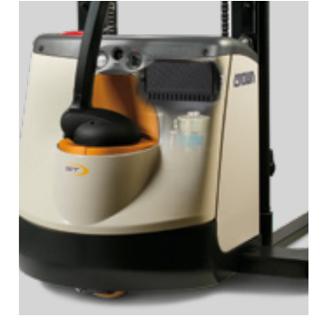
30 amp on-board charger
