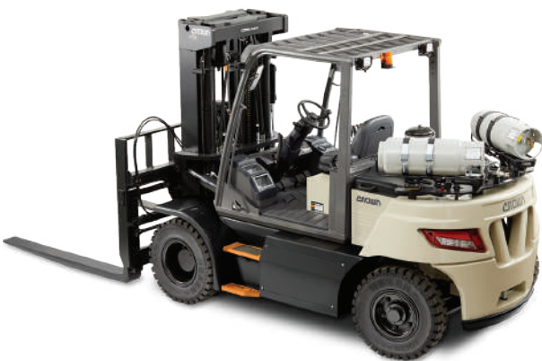
C-G Series, 50-70G Tyre: Cushion, Pneumatic Power: Internal Combustion - Diesel Load Capacity: 5000 to 7000 kg Lift Height: 2495 to 6050 mm
