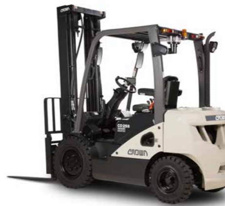
C-D Series, Model CD 20-30S Tire: Pneumatic Power: Internal Combustion - Diesel Load Capacity: 2000 to 3000 kg Lift Height: 2030 to 6500 mm
