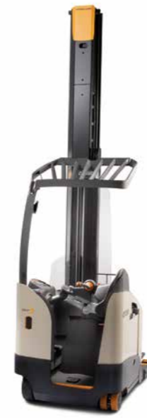
RM 6000S Series Load Capacity: 2000 kg Lift Height: 4875 to 12825 mm
