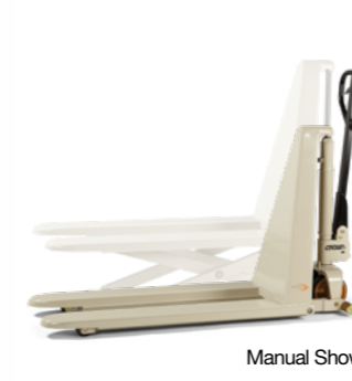
PTH 50S Manual Scissor Lift PTH 50PS Powered Scissor Lift Hand Pallet Truck Load Capacity: 1000 kg Lift Height: 800 mm
