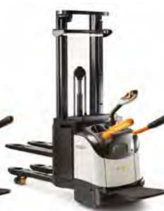
ET 4000 Series Rider Pallet Stacker Load Capacity: 1200, 1400 and 1600 kg Lift Height: 2440 to 5400 mm
