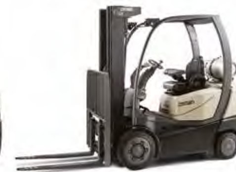
C-5 Series 4-Wheel LPG Counterbalance Truck with Cushion tyres Load Capacity: 2000, 2500 and 3000 kg Lift Height: 2665 to 7465 mm
