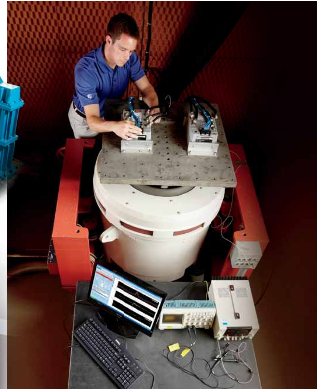
▲ An electrodynamic shaker qualification test applies 8,000 pounds of force to the product to ensure it withstands repeated impacts and vibration.
