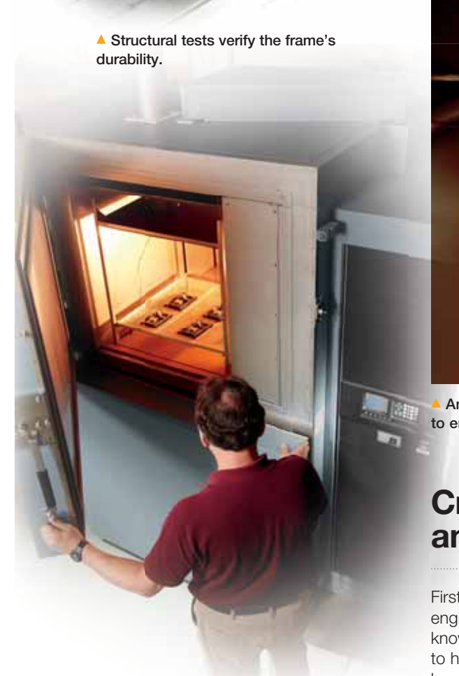
▲ Electrical components on our lift trucks are tested at -40° to 85°C to verify longevity in extreme temperatures.
