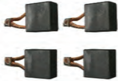
Part Number - 370274 Brush Set (Set of 4) 0.625 D x 1.240 W x 1.305 L
