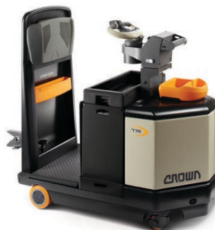
RT 4000 Series Rider Pallet Truck Load Capacity: 4,500 lbs. Forks: Double length available
