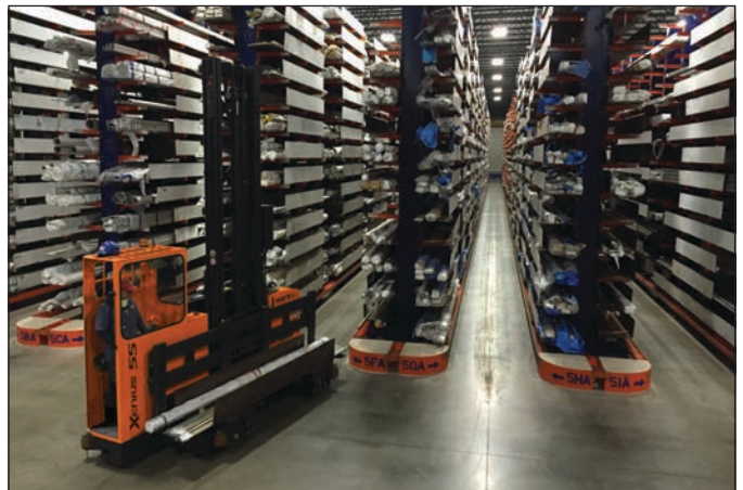
XENIUS - up to 12,000 lbs | up to 360" lift height
