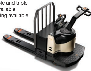
PR 4500 Series Rider Pallet Truck Load Capacity: 6,000 - 8,000 lbs. Forks: Double and triple lengths available
