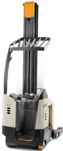
RM 6000 Series Load Capacity: 4,500 lbs. Max. Lift Height: 400 in.
