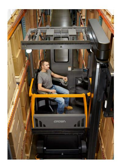
For example, the Crown RC Series of stand-up forklifts employ a contoured, low-profile power unit on the side where the operator is positioned to provide increased visibility during travel and a clear view of the forks when handling loads. Similarly, newer stockpickers feature expanded views through the platform window and on each side to facilitate order picking at height.
