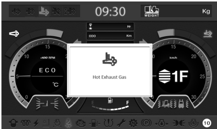
Display that notifies the operator of automatic DPF regeneration / SCR cleaning
