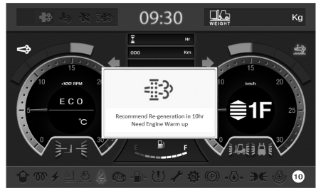
Display that notifies the operator of automatic DPF regeneration / SCR cleaning
